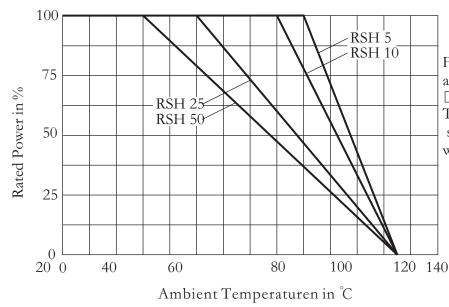
For resistors mounted onto heatsink and thermal resistance of 1  $^{\circ}$  C/W.
