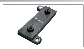
Manufactured in cermet thick film technology, these power resistors exhibit remarkable characteristics and the series includes 4 types ranging from 5 W to 50 W. Designed to be mounted onto a heatsink, the resistor can bear high short time overloads and 3 types of terminations are available. The resistors are non inductive and are particularly suitable for high frequency operation and cut-out circuits.
